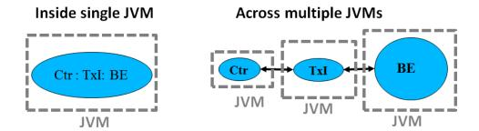
There is always exactly one Controller component and at least one Backend. Each Backend has one or more dedicated Transaction Injector(s) mapped to it. This logical mapping is called a "Group". The topology for a Group can be defined using command line options in the run script.
